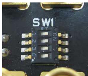
Figure 4: Photograph of the user switches
